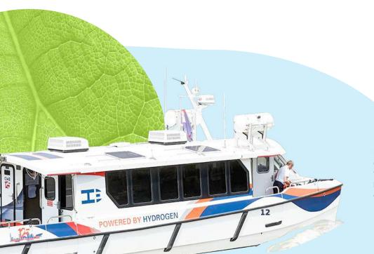
Hydroville is the first certified passenger vessel that uses hydrogen to power a diesel engine, Antwerp, Belgium.
